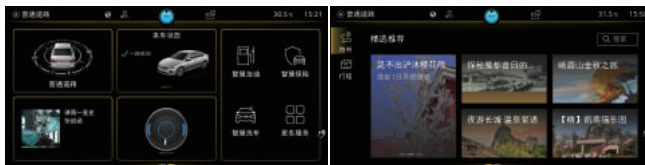
In-vehicle infotainment system: Dual OS system of Linux + Android
